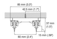
Extra Ceiling Double Bracket Bracket width = 23 mm (.91")
